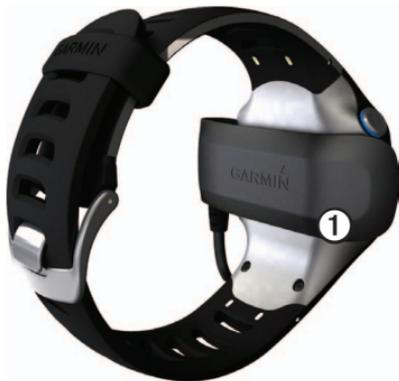
When you connect the Forerunner to a power source, the Forerunner turns on, and the charging screen appears.
